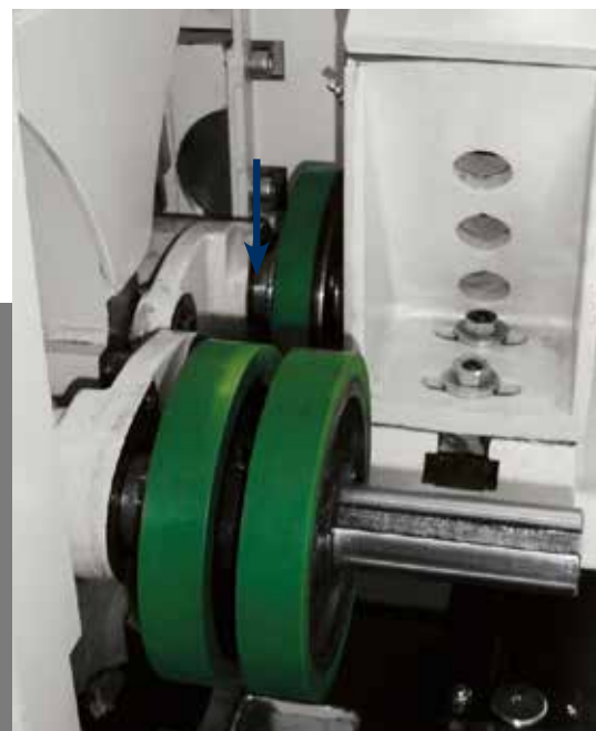
Feed unit placed after top horizontal spindle
