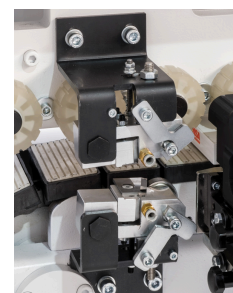
Glue Scraper station w/ floating blades
