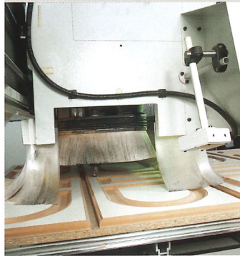
Digital camera - continuous precision control and monitoring of the working area
