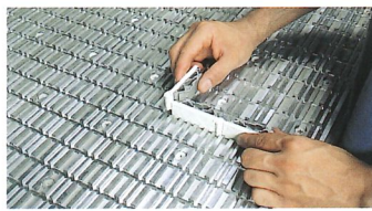
Easy worktable tooling. With three types of MPS suction cup, the practical MODULSET modular hold-down system and extra, electro pneumatically controlled perimeter stops
