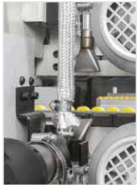
ID 3000 edge brightening unit It brightens the colour of plastic edges by heating them with hot air.
