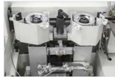
RT-V1 premilling unit A perfect panel surface for an excellent joint line.
