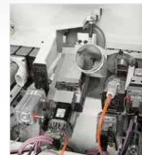
R-HP Trimming-Chamfering unit Quick changeover between 2 different radii, infinite thin edges and solid wood tipping thanks to Multiedge devices.
