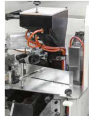
SGP-E glue pot Perfect joint line and use of EVA and PUR glue.
