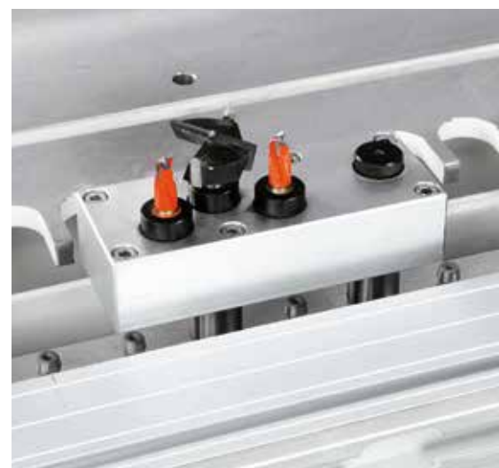
Hinges units For increased versatility, the quick change chucks can be fitted with various types of bits for different operations, like drilling hinges locations.
