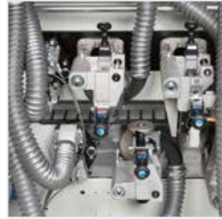
RAS-V edge scraping unit: perfect radius on plastic edges.
