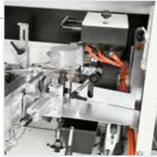
SGP-E glue pot: homogeneous application of the glue on all materials.
