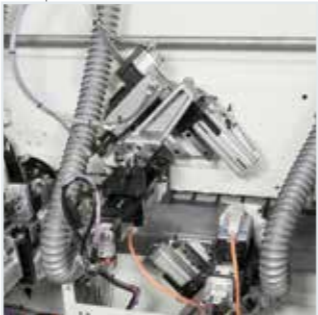
ROUND X MULTIEDGE rounding unit with 2 motors and NC axes for an automatic set up.
