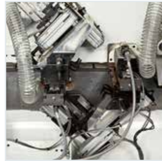
ROUND X 2-motor rounding unit: excellent quality of the panel with simultaneous rounding and trimming of the edge.
