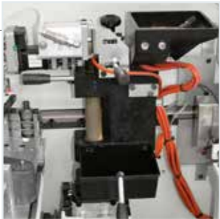
Perfect junction line and use of EVA and PUR glue thanks to "SGP" glue pot.
