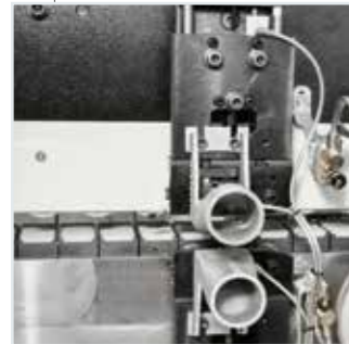
RC-N glue scraping unit: It eliminates any excess of glue in the joint between panel and edge.
