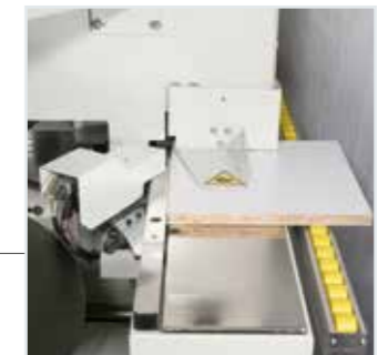
Easy size: infeed guide with axis for the NC adjustment of the material removing of the pre-milling unit.
