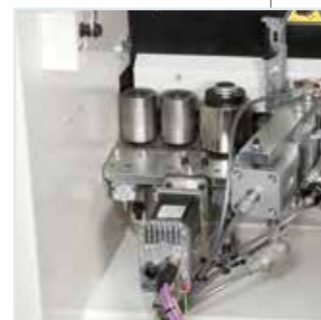
Pressure roller conveyor with electronic positioning and timed intervention.
