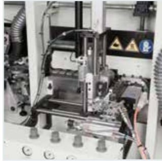
ROUND 1 rounding unit: rounding of corners on straight and shaped panels.
