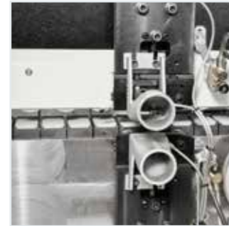
RC-N glue scraping unit: it eliminates any excess of glue on the panel/edge junction. Nesting machining.
