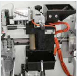
Perfect junction line and use of EVA and PUR glue thanks to the "SGP" glue tank.
