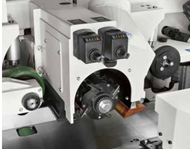
Kit to enable the profiling of the top horizontal spindle It includes n.2 mechanical readouts with decimal precision. Min./max. tool diameter: 100/180 mm. Axial stroke: 40 mm.
