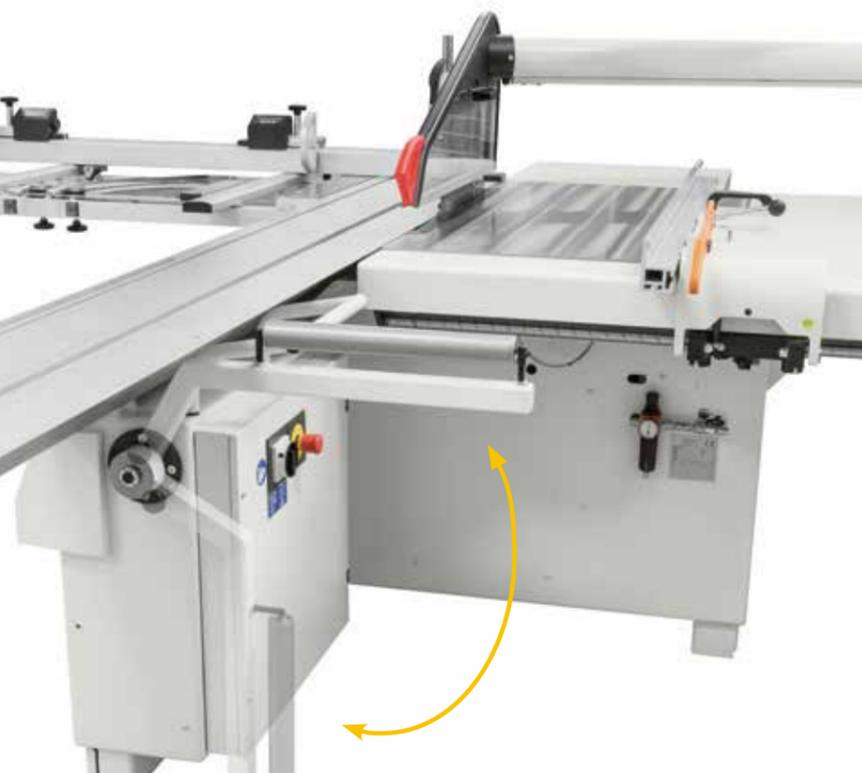
**Extension with roller conveyor on parallel fence side,**
