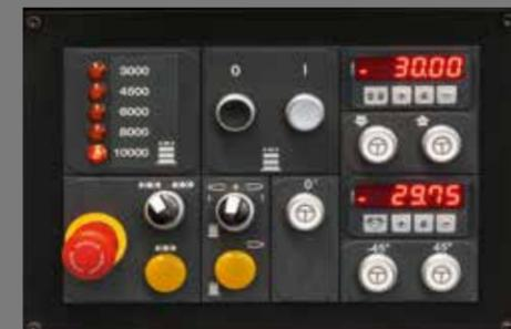
**Powered operating unit movement with digital readouts.**
