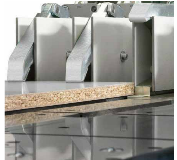
CLAMPS WITH SELECTIVE CLOSING (optional): this device prevents ruining panels which edges are exactly positioned in correspondence of the clamps working area.
