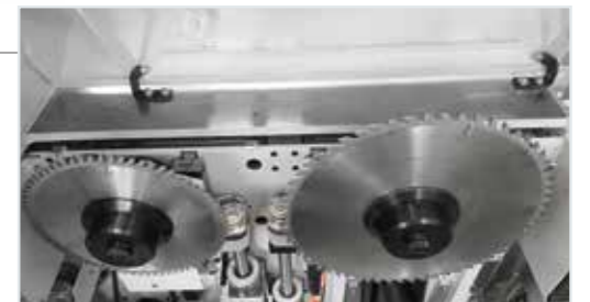
Hi-Tronic vertical stroke device: top of productivity with the new saw carriage (optional).
