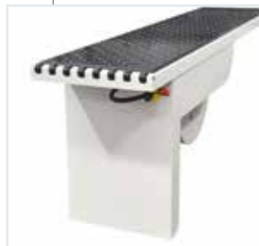
Selectable air blowing table: an essential tool Possibility to enable/ disable the air blowing feature on each table section via four independent motors. It ensures optimal sliding of the panels only where it is needed and avoids the accidental falling of panels already cut and temporarily stored on the tables.
